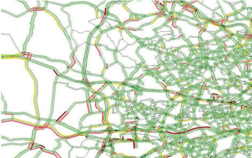
Figure 4-25: PM Peak 2031 Do Something Volume Over Capacity on links as %
