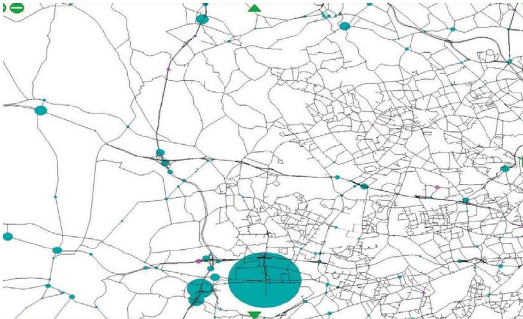
Figure 4-28: PM Peak Optimisation – Change in Junction Delay (Scenario B – Scenario A)
