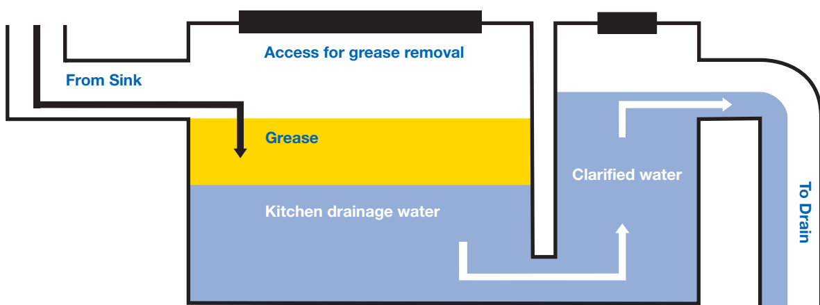
Diagram of an "under-the-sink" grease trap
